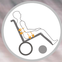
▲ Pressure is distributed when using tilt-in-space
